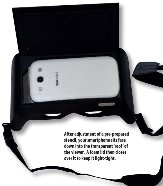
After adjustment of a pre-prepared stencil, your smartphone sits face down into the transparent 'roof' of the viewer. A foam lid then closes over it to keep it light-tight.
