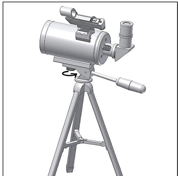
Figure 4. Use the hand knob to fix the tube.
