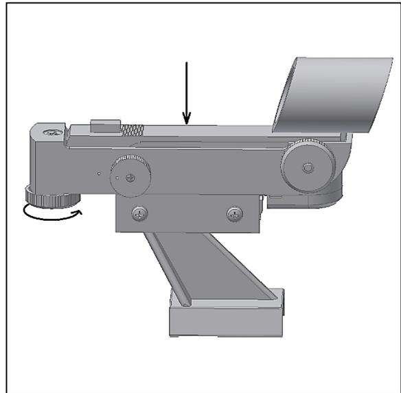
Figure 7. Turn altitude adjustment knob to align finder.
