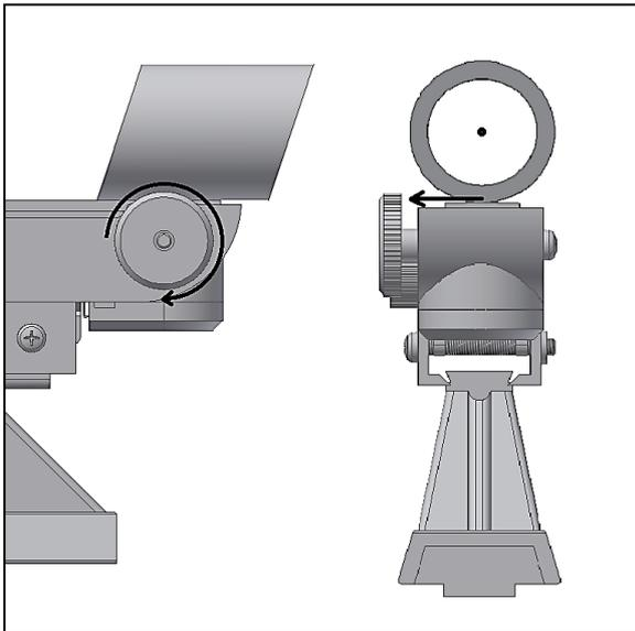
Figure 6. Turn azimuth adjustment knob to align finder.
